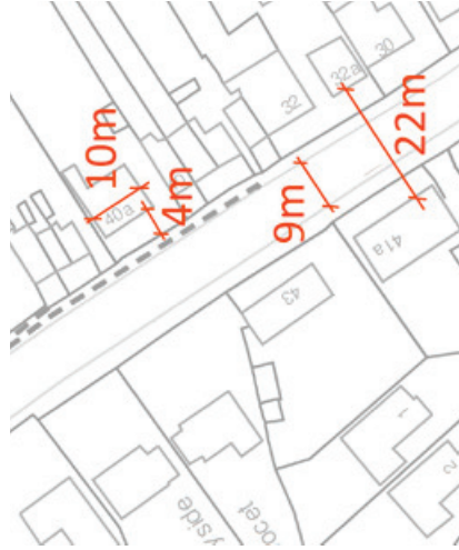
Fig 4.2.7 Key relationships and geometries for assembling a representative section of Lincoln Road. Wide streets allow for verges and pavements, and plots have room at the front for a decent garden.
